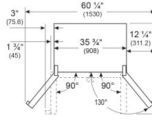
Drawers can be pulled out with door open to 90°. Drawers can be taken out with door completely opened.
