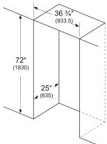
Leave 2" (50.8) gap at the top and 1 %" (34.9) behind the refrigerator for proper ventilation.
