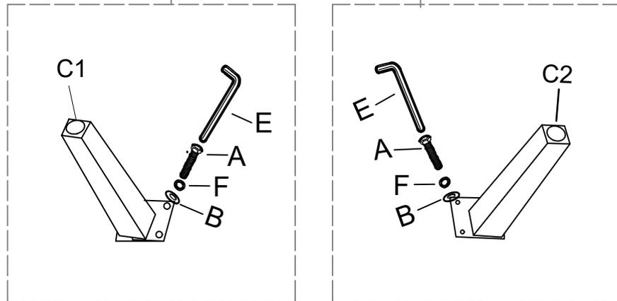
Do not fully tighten until all bolts have been inserted.
