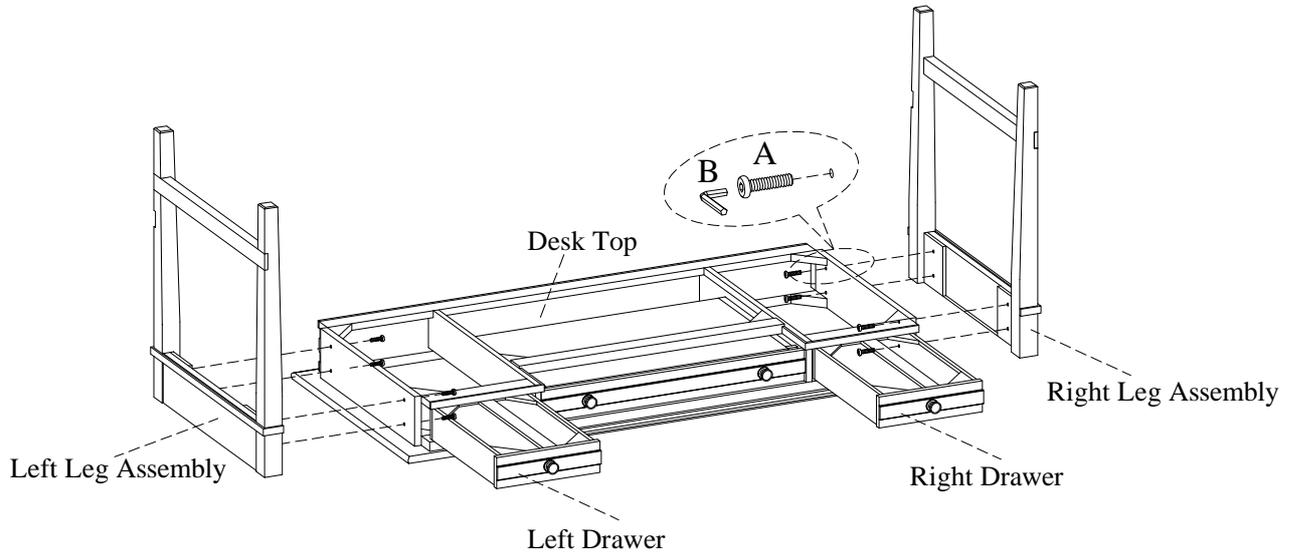
**STEP 3:** Attach the back stretcher using 2 bolts (A). Then use the Allen wrench to tighten all bolts. Push back the left & right drawer boxes, and return the desk to the upright position.
