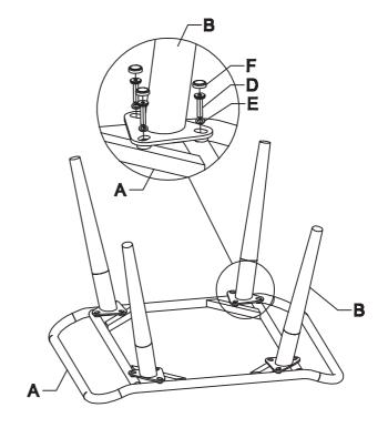
2.Pls secure screw all the bolts are tightened completely, four for each leg, totally 12pcs bolts, if you find the bolts can not be screwd tightenly ,pls return the chair.
