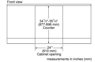
Thermador double drawer under counter top dimension. (Unit door flushed with the cutout) measurements in inches (mm)
