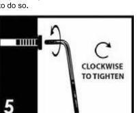
Make sure all parts are properly aligned, then use the appropriate hand tool to completely tighten the bolts or screws. Do not use power tools and do not overtighten.
