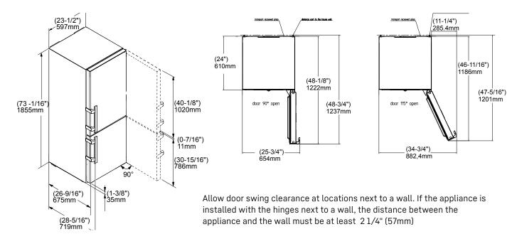
The refrigerator door must open to a minimum of 90° to allow the crispers to open and the shelves to be removed. There is no 90° door limiter available for this model.
