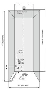
The appliances can be used freestanding or semi built-in. If semi built-in, consider the minimum cabinet opening dimensions specified on this image. For ventilation requirements, please follow instructions on section Ventilation
