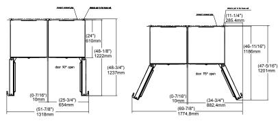
If the appliances are installed with the hinges next to a wall, the distance between the appliance and the wall must be at least 2 1/4" (57mm). This is how far the handle protrudes when the door is open. A set for restricting the door opening angle to 90° can be acquired from Customer Services for appliances with soft closing. For detailed measures for each appliance, see product page on this guide
