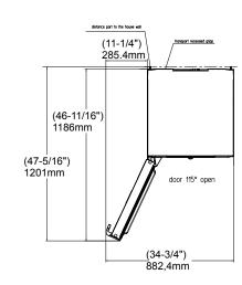
Allow door swing clearance at locations next to a wall. If the appliance is installed with the hinges next to a wall, the distance between the appliance and the wall must be at least 2 1/4" (57mm)
