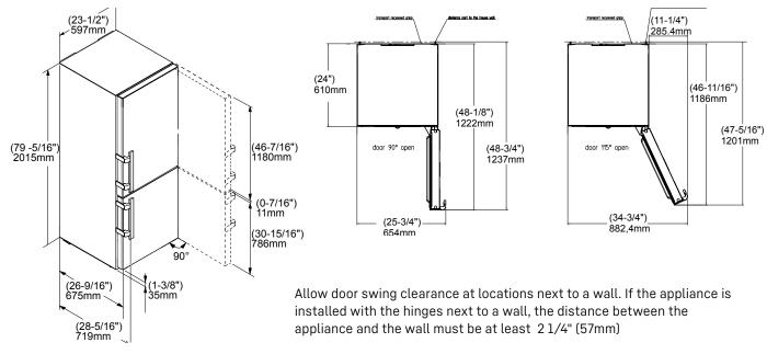
The refrigerator door must open to a minimum of 90° to allow the crispers to open and the shelves to be removed. There is no 90° door limiter available for this model.
