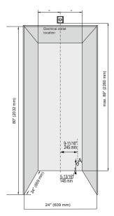
The appliances can be used freestanding or semi built-in. If semi built-in, consider the minimum cabinet opening dimensions specified on this image. For ventilation requirements, please follow instructions on section Ventilation
