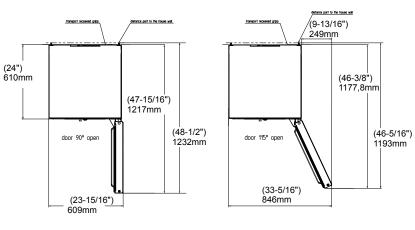
Allow door swing clearance at locations next to a wall. If the appliance is installed with the hinges next to a wall, the distance between the appliance and the wall must be at least 1/2" (13mm)
