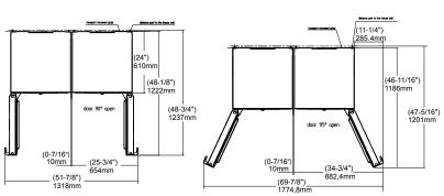
If the appliances are installed with the hinges next to a wall, the distance between the appliance and the wall must be at least 2 1/4" (57mm). This is how far the handle protrudes when the door is open. A set for restricting the door opening angle to 90° can be acquired from Customer Services for appliances with soft closing.
