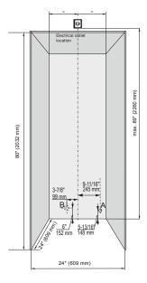
The appliances can be used freestanding or semi built-in. If semi built-in, consider the minimum cabinet opening dimensions specified on this image.
