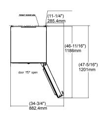
Allow door swing clearance at locations next to a wall. If the appliance is installed with the hinges next to a wall, the distance between the appliance and the wall must be at least  $2 \frac{1}{4}$  (57mm)
