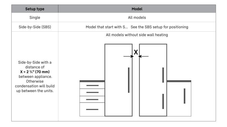
Only specific models can be combined for a side by side installations keeping always the original door opening, as they include a heating blanket in the opposite side of the handle to avoid condensation when attached together:
