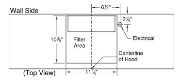
A minimum of 25 sq. in. of exhaust opening space per blower/filter assembly, located above the filter assembly outlet (top), is required for proper air recirculation.
