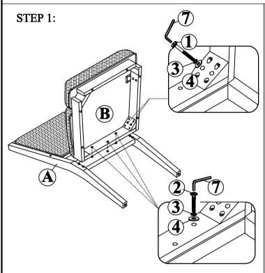
Step 1: Place Chair Back (A) on the floor. Attach Seat Box w/Seat Cushion (B) to the Chair Back (A) by inserting Big Flat Washer (4), Lock Washer (3), Long Bolt (1) into the holes at the rear corner block of the Seat Box w/Seat Cushion (B) and secure by Allen Key (7). Insert Big Flat Washer (4), Lock Washer (3), Short Bolt (2) into the rear bar of the seat frame. Tighten all bolts by Allen Key (7). Do not fully tighten.
