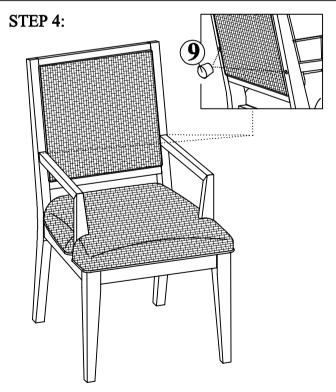
Step 4: Place Arm Chair on flat surface and adjust chair legs until level and chair does not wobble. Fully tighten all Bolts and Hex Nuts at this time. Insert Wood Plug (9) into the holes on Chair Back (A) as the picture shown.
