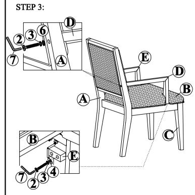
Step 3: Turn the Arm Chair to upright position. Attach the LSF /RSF Arm (D/E) to the Seat Box w/Seat Cushion (B) by using Big Flat Washer (4), Lock Washer (3), Short Bolt (2) and tighten with Allen Key (7).
