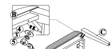
Step 2: Attach Front Leg (C) to the Seat Box w/Seat Cushion (B by inserting Big Flat Washer (4), Lock washer (3) and Hex Nut (5) through the bolts and secure by Hex Wrench (8). Do not fully tighten.
