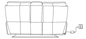
STEP 3 - Connect the connector from motor to the power cord and transformer
