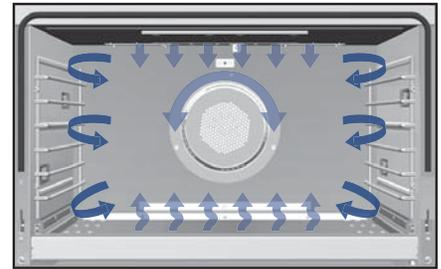
When roasting using this setting, cool air is quickly replaced, searing meats on the outside and retaining more juices and natural flavor on the inside with less shrinkage.
