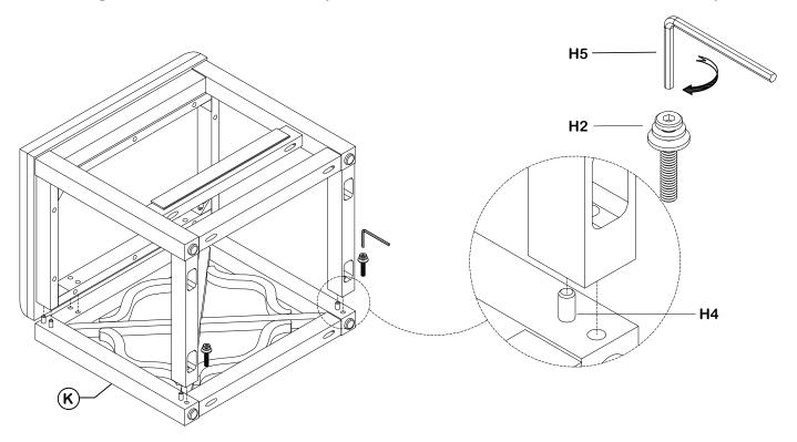
STEP 8 ( x1) Do not over-tighten the bolts. Make sure you use the lock washers to ensure the bolts stay fastened
