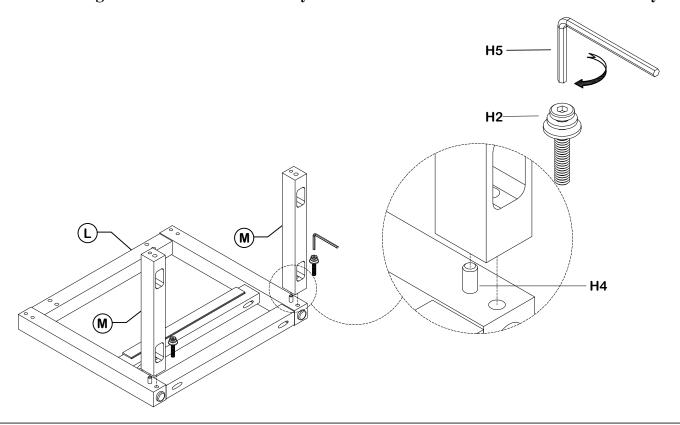
STEP 6 ( x1) Do not over-tighten the bolts. Make sure you use the lock washers to ensure the bolts stay fastened
