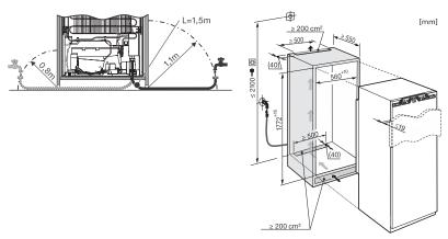
FNS37492iE, KFN37692iDE, KFSN37692iDE, Water connection placement 2013 (installation drawings)
