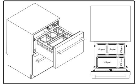
2. Install the pans into your preferred sections. The 1/9 pan must be accompanied with two 1/6 pans or one 1/3 pan for a proper fit.
