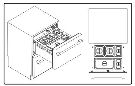
3. Install the pan lids onto their correct sized pans.
