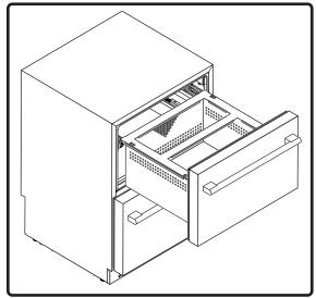
1. Open the upper drawer. Place and align the stainless steel pan support bracket onto the rims of the drawer.
