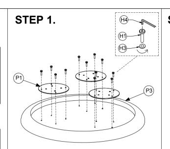
\*Screw the bolts out to take frame out (P1) of top (P3)
