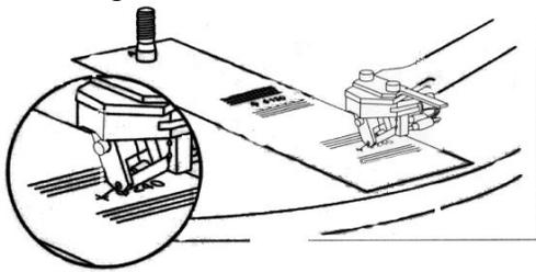
**VTA Adjustment:** The VTA for the installed Goldring cartridge has been properly set at the factory. To adjust the VTA for other cartridges, lay a record on the platter (5). Slacken the horizontal adjustment screws (two **Allen** screws located near the plinth on the back of the tonearm pillar) with the Allen Key provided.
