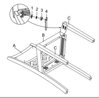
STEP 3 Place the assembled seat frame on the cushion seat and attach with wood screws.
