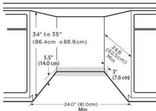
\* Make sure water line, wires and drain hose are within the shaded area.
