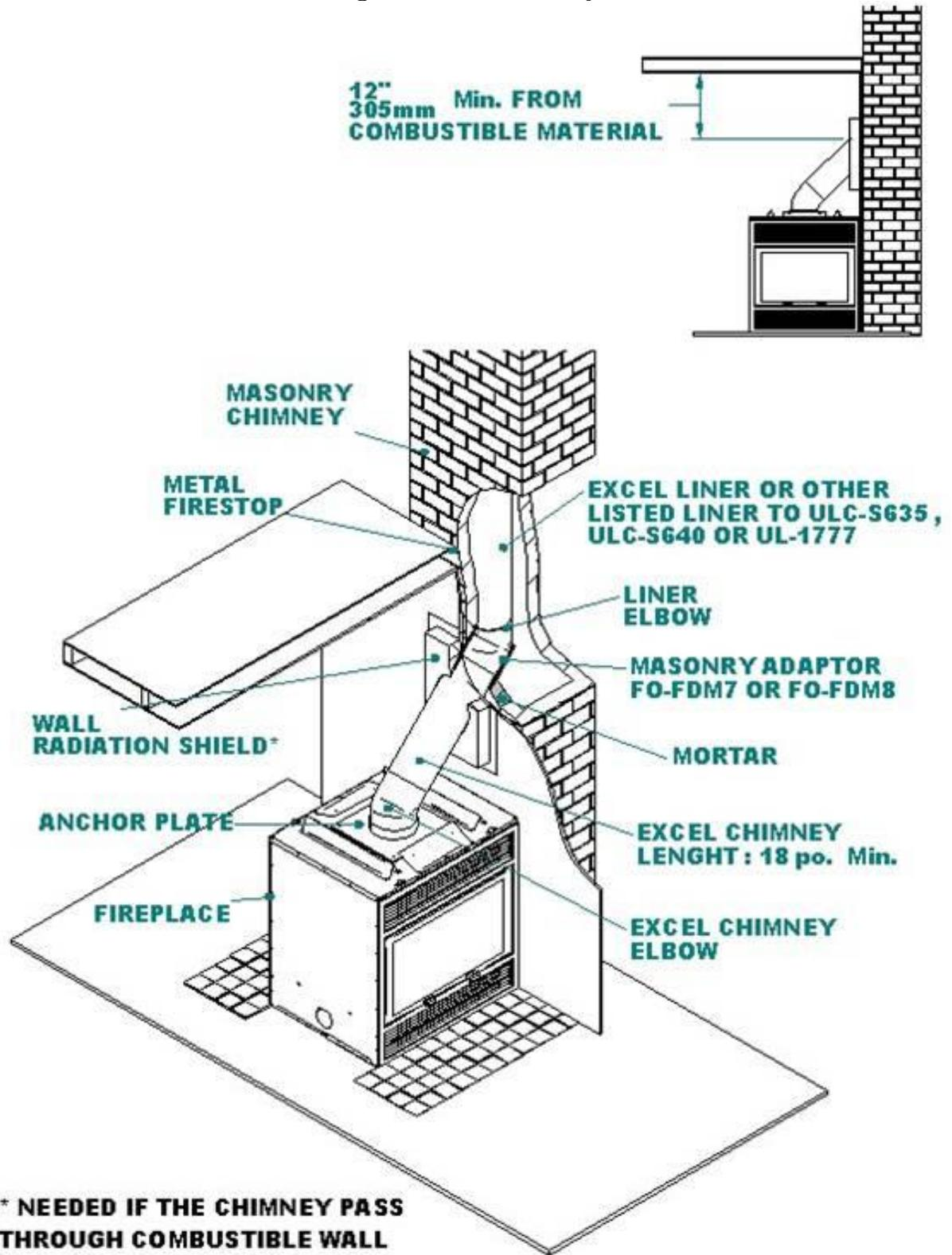
Figure #7: Straight Chimney Installation
