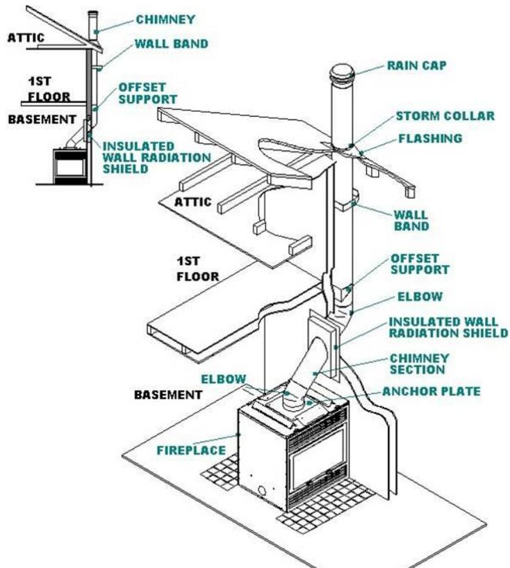
Figure #10: Minimum Chimney Height
