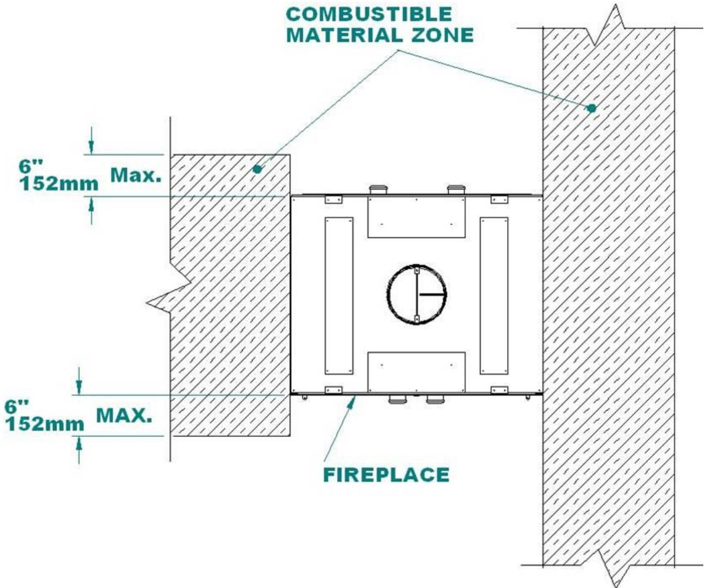
Figure #12: Chimney Enclosure
