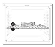
If the level doesn't show that the rack is level, adjust the leveling legs with a wrench.
