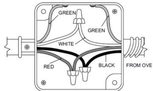
5. Connect the 2 black wires together using a UL listed wire connector.
