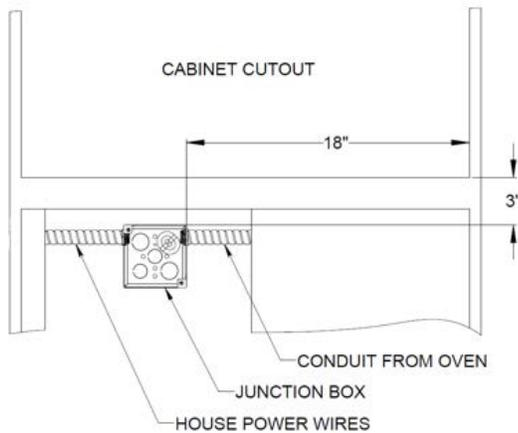
3. Move the oven with flexible conduit/wires close to the cabinet cutout and feed the wires and conduit through the rectangular cutout located at the rear end of the cabinet cutout base.
