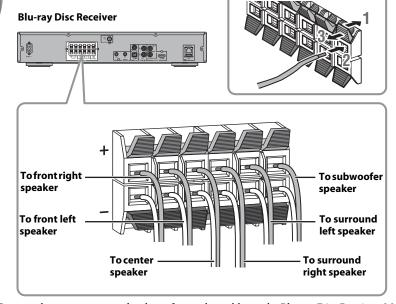
Connect the center, surround, subwoofer speaker cables to the Blu-ray Disc Receiver, Make sure you connect the speakers with the correct polarity: positive (+) cables to positive (+) terminals, and negative (-) cables to negative (-) terminals.
