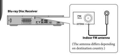
Connect the supplied indoor FM antenna to the Blu-ray Disc Receiver, as shown. See the owner's manuals for more information about connecting an antenna.
