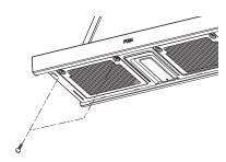
To remove, slide the grease filter forward slightly and pull it downward.
