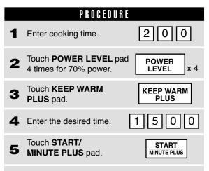
The operation will start. When the cooking time is complete, a long tone will sound and Keep Warm Plus will start. The display will count down for 15 minutes and KEEP WART will be displayed during the count down.
