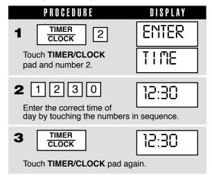
This is a 12 hour clock. If you attempt to enter an incorrect clock time, ERROR will appear in the display. Touch the **STOP/CLEAR** pad and re-enter the time.
