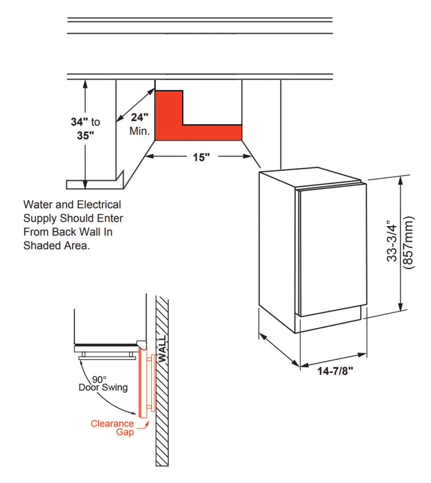
When installing with the hinge side next to a wall, leave adequate space for your door handle.
