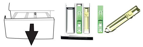
Press the dotted point on the siphon of the softener compartment and pull towards yourself until the it is removed from the dispenser.
