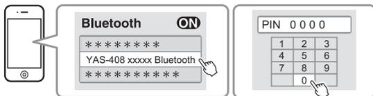
When the connection between the Bluetooth device and the unit is established, a completion message is displayed on the Bluetooth device, and the
