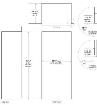
NOTE:  $3^{1/2^n}$  (89) finished returns will be visible and should be finished to match cabinetry Shaded line represents profile of unit.
