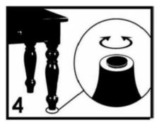
Some furniture comes with height adjustment knobs underneath each leg. To lower or to raise each leg, you need to turn clockwise or counterclockwise, respectively.
