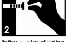
Position each part correctly and insert screws or bolts into their respective holes by hand tighten or using the proper hand tool. Only tighten when step is completed or when instructed to do so.
