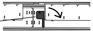
To keep the table closed, lock the rails on each side of the table.
