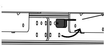
To open the table, unlock the rails on each side of the table.
