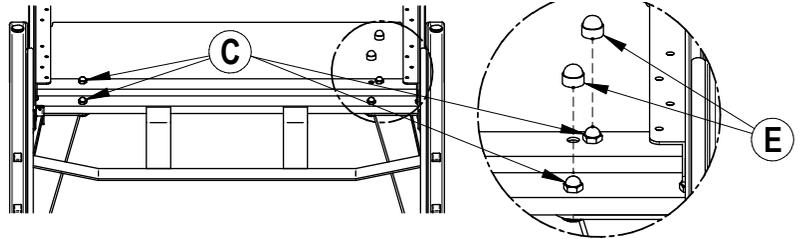
4) Put the table top upside down on a large blanket to protect its finished surface. Put the base frame 1 on the table top. Center base frame and align rail holes with pre-drilled holes in the table top.
