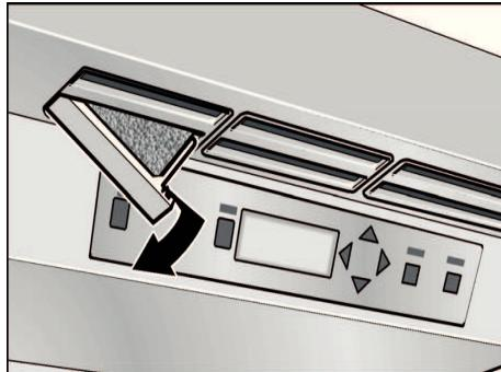
2. Remove the used filter and replace with a new one.
