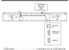
**OPTICAL IN** ...... Connect to an optical device.
