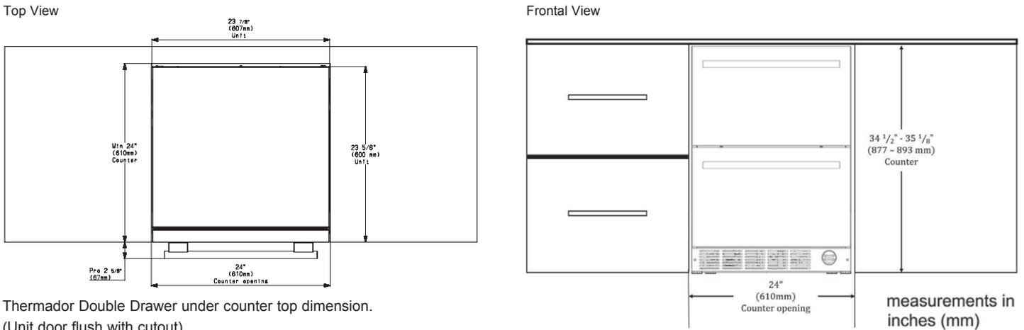
Thermador Double Drawer under counter top dimension. (Unit door flush with cutout)
