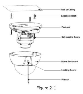
**Step 1** Use the wrench in the accessories bag to unscrew the three torx head screws on the dome enclosure and then open the dome enclosure.
