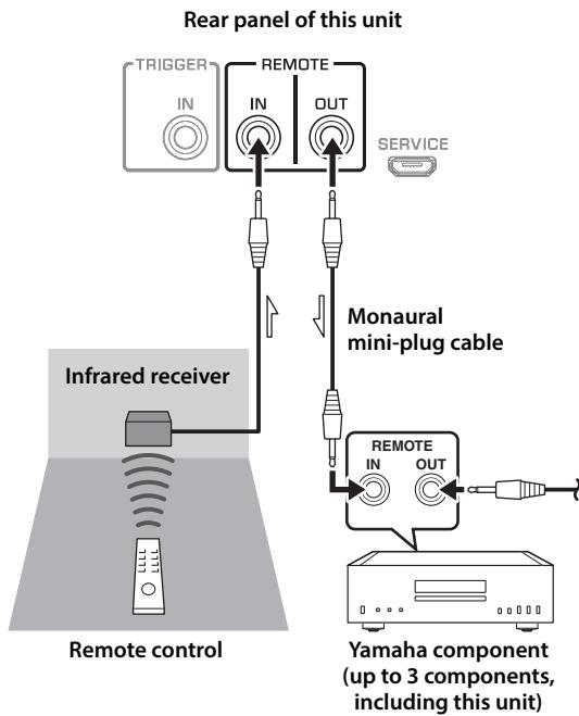
After all connections are complete, plug the power cable into the AC IN connector of the unit, and then plug the power plug into the AC outlet.
