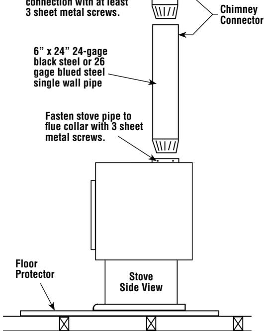
**Figure 5 - Typical Installation**
