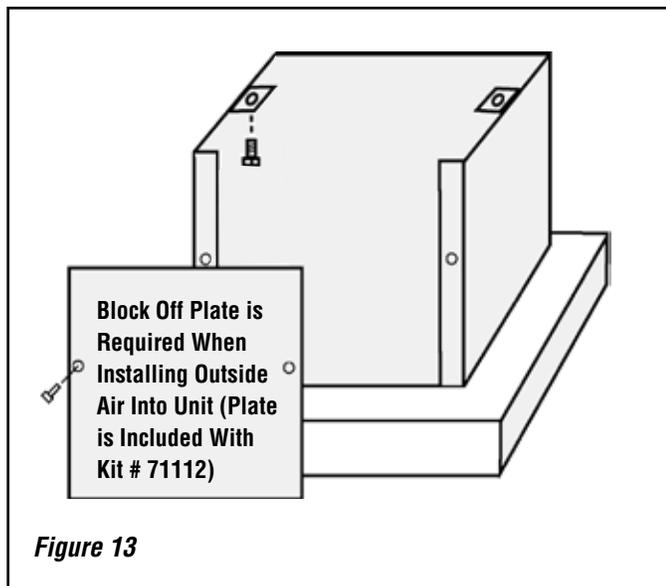
5. If required, install the Outside Air Kit (cat. no. 71112) as per the following instructions. To locate the hole in the hearth for outside air mark and cut a 4" (102 mm) hole in the hearth. The hole's center should be 3" (76 mm) directly forward from the center of the flue outlet or locate as per the instructions below.
