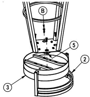
6) Center 3 seat on belt of 2 backrest and tighten firmly all B bolts.
