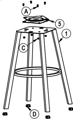
4) Bolts-on 5 swivel plate on 1 stool base with A bolts and C nuts.
