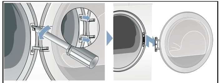
3. Place the door on a flat, smooth, secure surface such as a towel or cloth lying on the floor or table.
