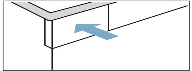
Ensure the tank is pushed back into the dryer until you feel it lock in place
