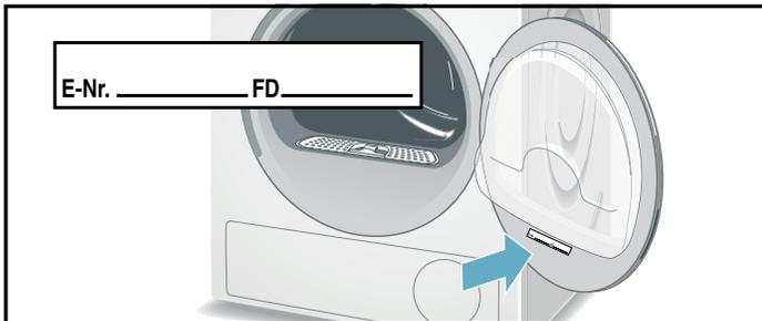
The **E-Nr.** (model number) and the **FD** (serial) number can be found on the rating plate label (shown above) or in the Home Connect application under Appliance Information.
