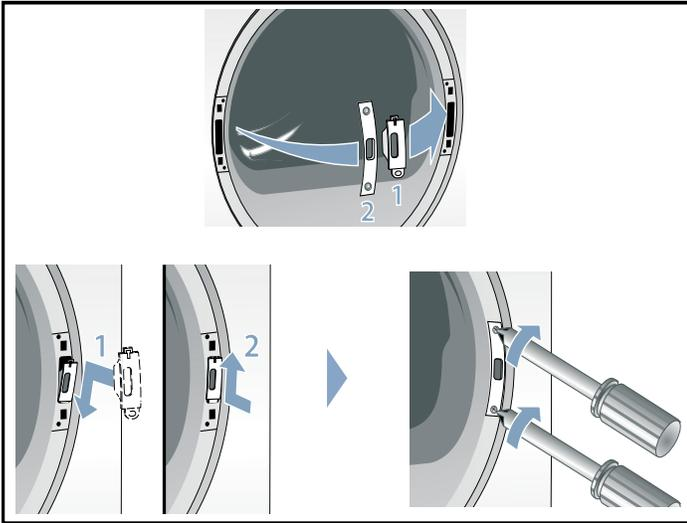
**13.** Install the door and hinge assembly back on the dryer with the original screws.
