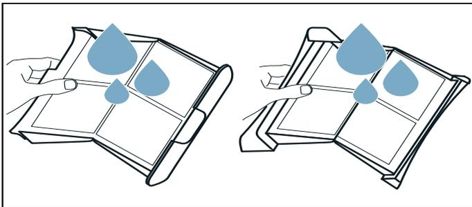
**NOTICE:** Both filters should be completely dry before putting them back in place in the dryer.
