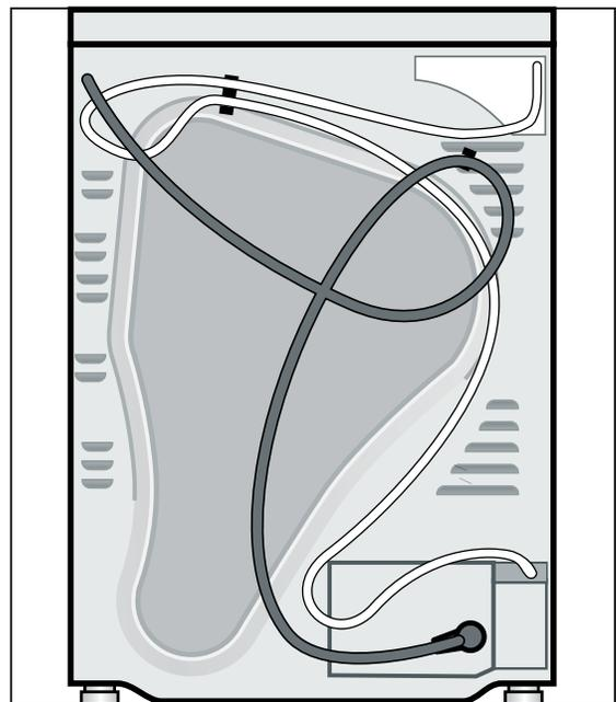
If you do not have a drain system or would like to use the tank to collect the condensate water for you to empty, follow the below instructions.
