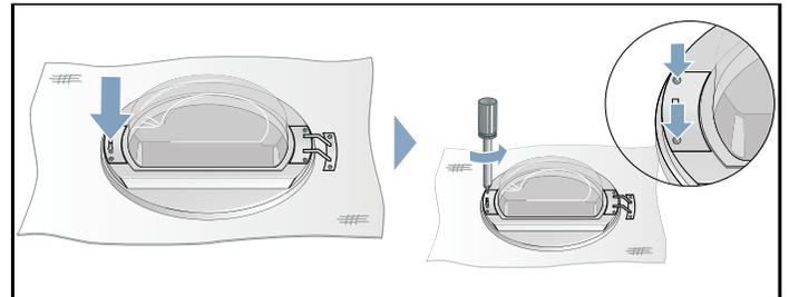
10. Remove screws from the door latch cover and then remove it from the dryer housing.
