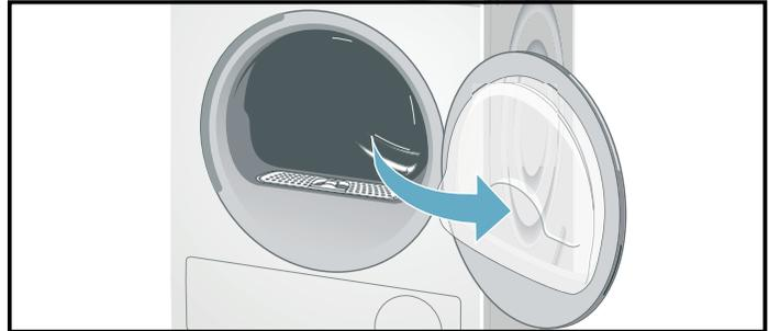
2. The deposit on the sensors can easily be removed by wiping the sensors (the two bars next to the lint filter) with a cloth and white vinegar.
