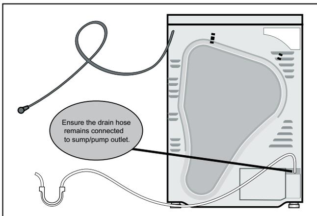
**NOTICE:** Do not reuse an old or different drain hose. Only use the drain hose included with the dryer.
