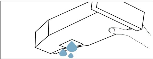
3. Take the blue filter from the Tank Kit and install it in the working position as shown in the picture below. Make sure it snaps completely in place.
