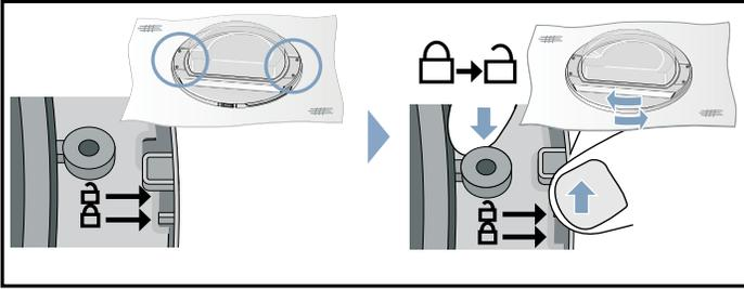
7. Separate the ring from the door body and rotate the ring 180° from its original position. Fit the ring back to the door body as shown below.
