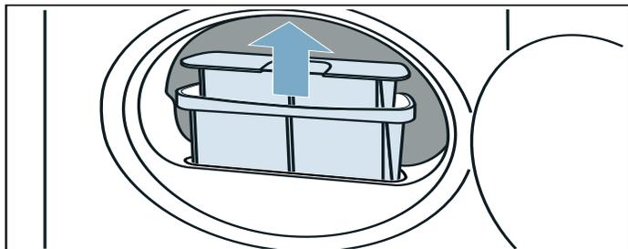
The filters should be cleaned after or before every drying process. Cleaning the filters reduces the drying time and saves energy.
