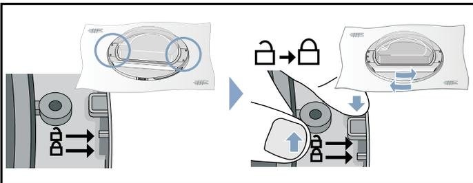
9. Place the hook insert in position adjacent to the handle slots/openings and the hinge insert in the opposite position as shown. Reinstall the original screws.
