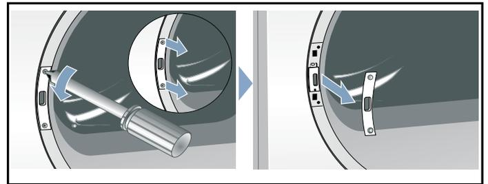
11. Remove the door latch from the dryer housing.
