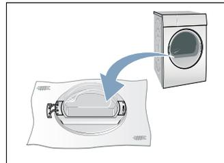
4. Remove screws from the hinge insert and then remove it from the door.
