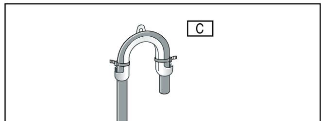
Secure hose and/or elbow as shown below. Sink "D" or floor "E".
