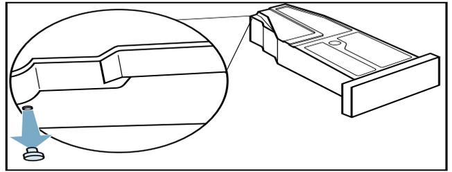
6. Check that both the blue filter and black plug are fully in their correct positions and insert the complete tank into its position in the dryer.
