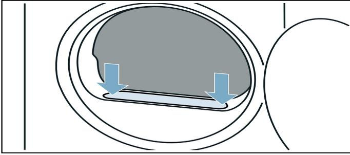
4. Separate the two-part lint filter and open both parts as shown.
