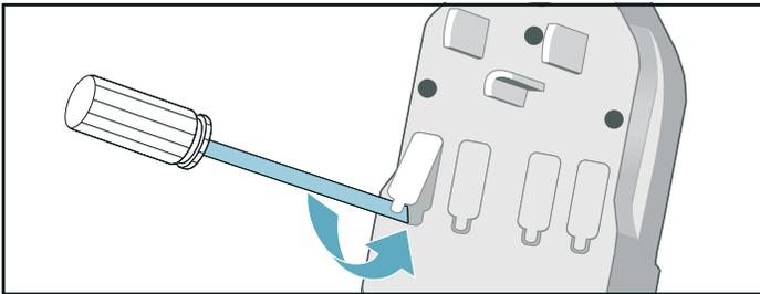
2. Remove fuse holder using a pointed tool as shown (e.g. pick or small screwdriver).
