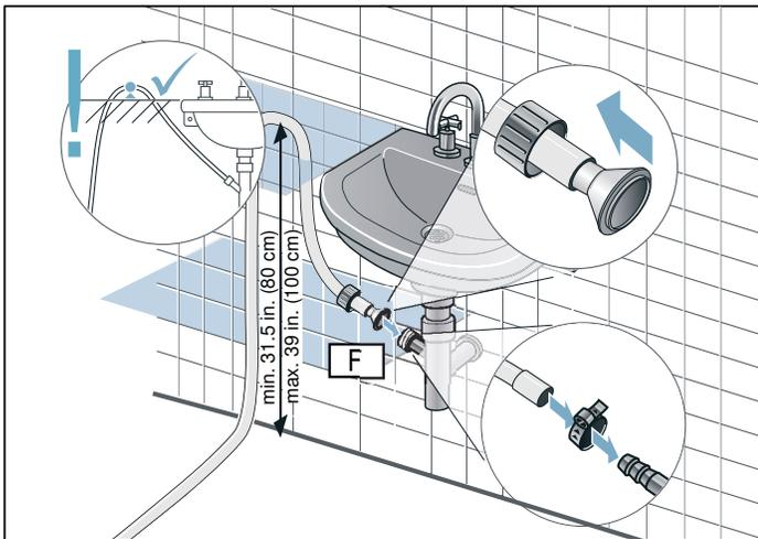
Minimum height of drain for installation shown above is 31.5 in. (80 cm). Maximum height of drain is 39 in. (100 cm).
