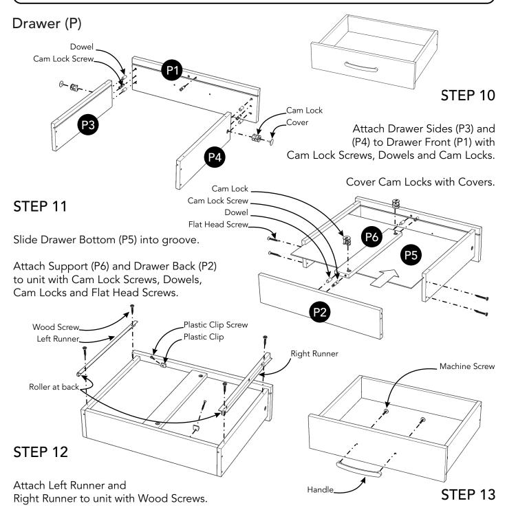
Attach Plastic Clips to unit with Plastic Clip Screws.
