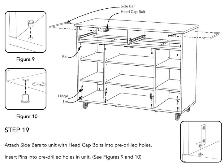
Insert Hinges into Pins. (See Figure 11)
