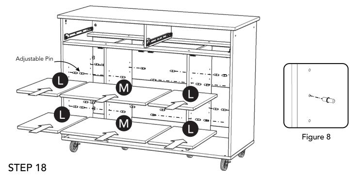
Insert Adjustable Pins into side panels and middle panels at desired level. (See Figure 8) Place Shelves (L) and (M) into position.
