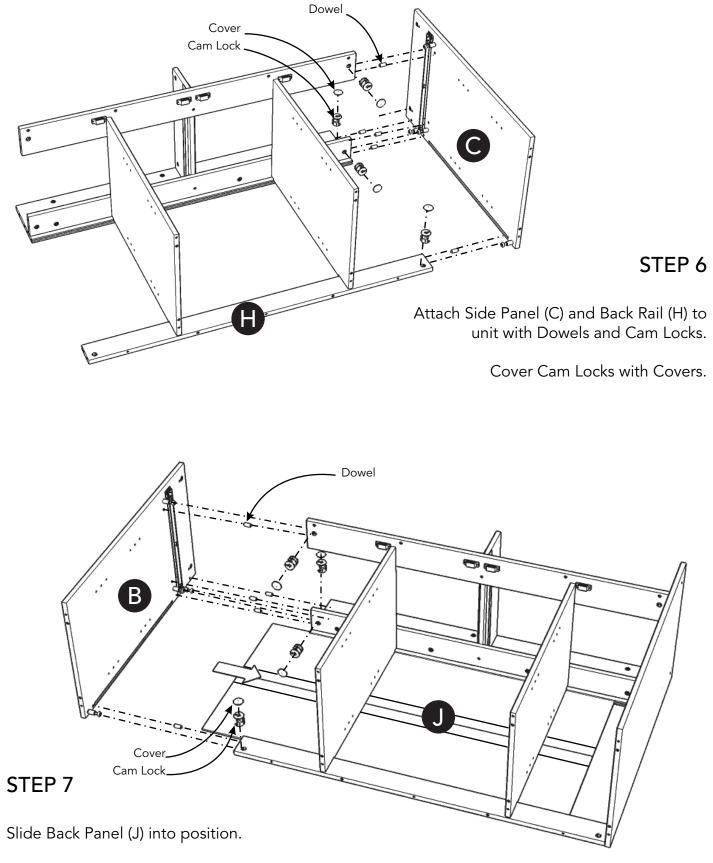
Attach Side Panel (B) to unit with Dowels and Cam Locks.
