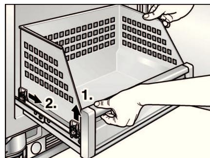
2. Lift tray at front slightly and insert into the runners.
