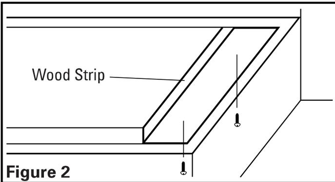
2. The thickness of the strips should be the same as the recess of the cabinet and they should be approximately 2" wide.
