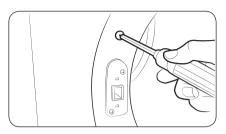
6. Remove the two screws above and below the lever holder on the opposite side of the door opening.
