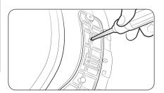
10. Insert the screw you just removed into the other screw hole on the back of the door hinge, and then tighten.
