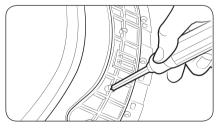
**9.** Remove the single screw from the back of the door hinge.
