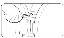
**11.** Place the door on the other side, and then reattach it to the dryer.
