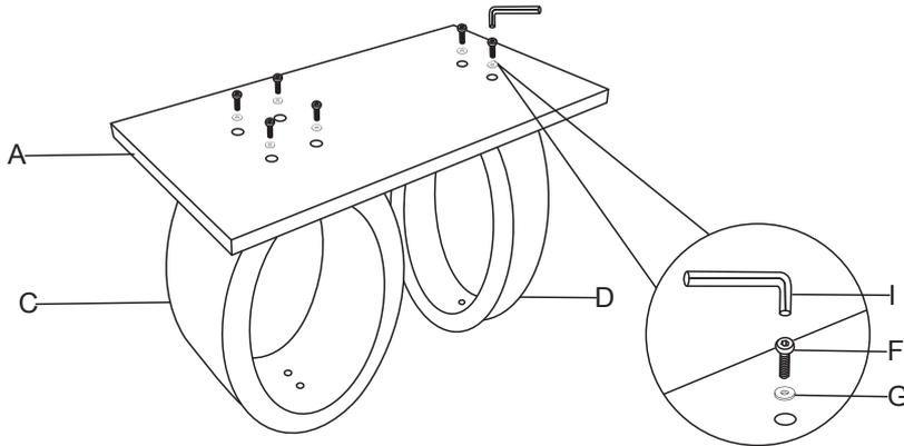
Firstly, fix the table leg with table base but do not fully tighten the bolt(F).
