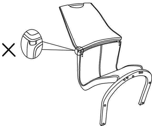
Step 2-a: Put the backrest (C) into the holes on the seat (B), press a little to make the screw holes on the backrest (C) align with the screw holes on the seat (B), lock these four holes with bolts (E). (Note: do not lock completely at this step)
