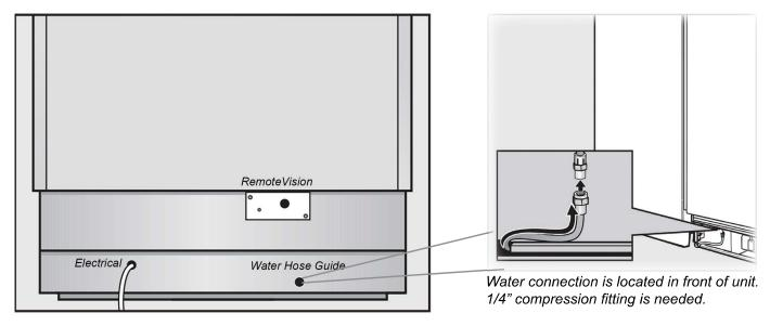
Electrical - 5 foot (1.52 m) - 120 Volt - 15 Amp - NEMA 5-15 molded plug Water line - 1/4" flexible water line - not included
