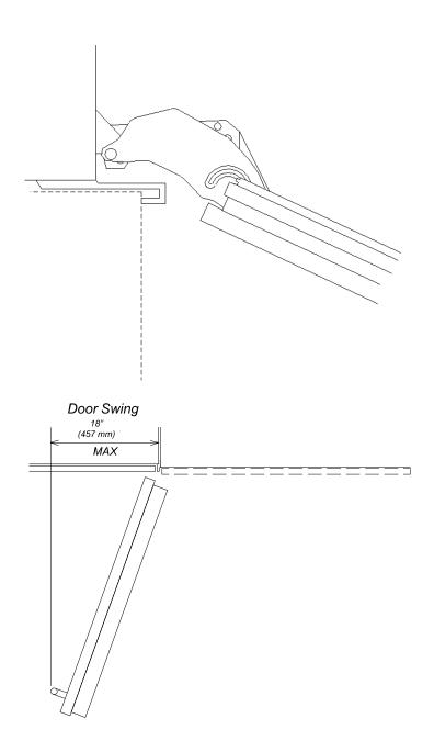
**NOTE**: Additional space needed depending on the thickness of front panels and handle used.
