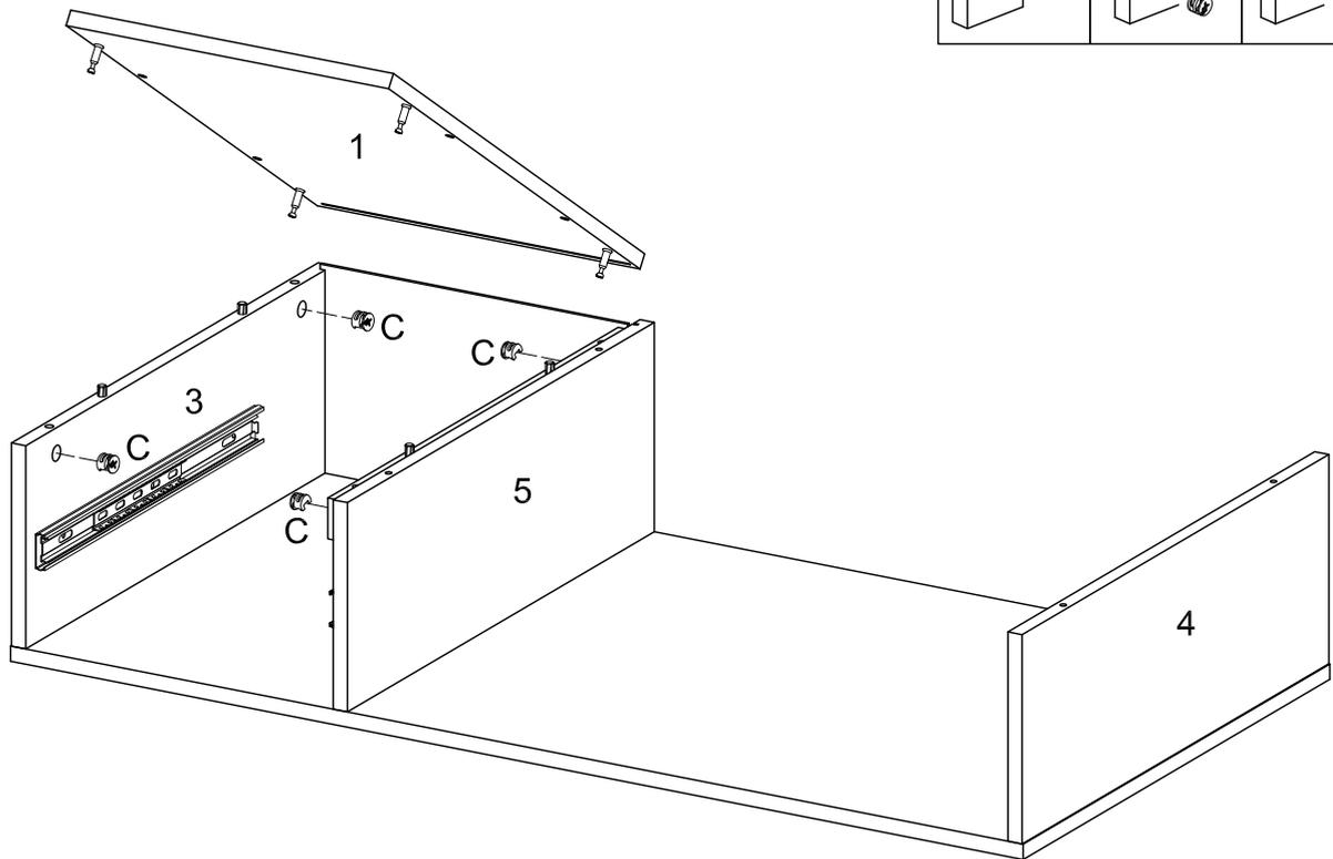
Insert top panel (1) into side panel (3,5), then insert and secure cam lock (C) to side panel (3,5) to lock it.
