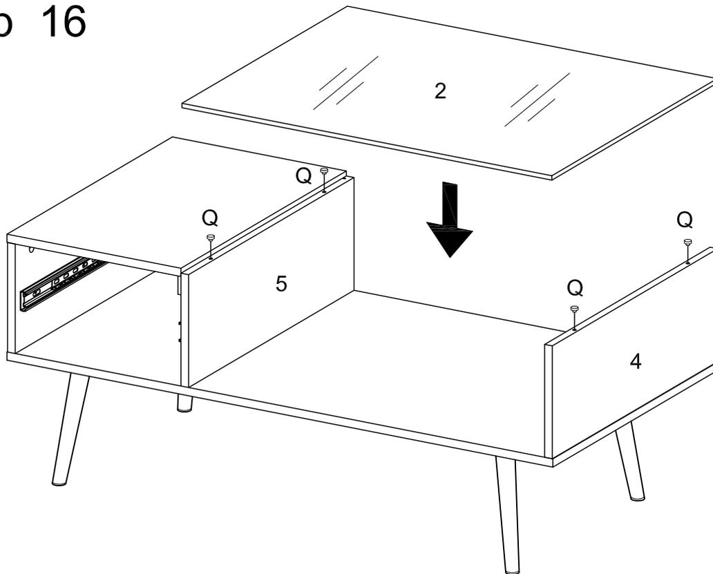
Place rubber suction cup (Q) over holes as per diagram, then place glass top on top of frame carefully.
