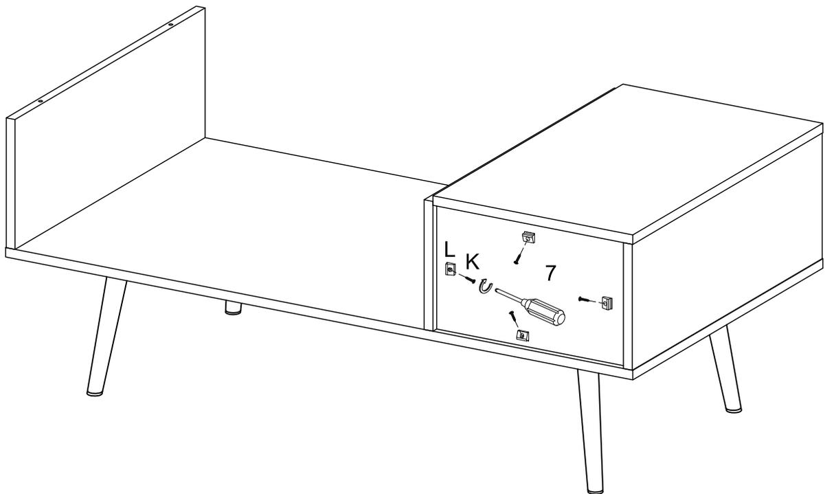
For optional added stability, secure plastic wedge (L) to back panel (7) with screw (K).
