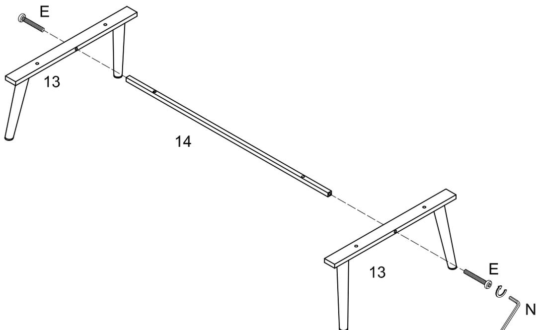
Use wrench (N) to secure leg (13) to part (14) with bolt (E).
