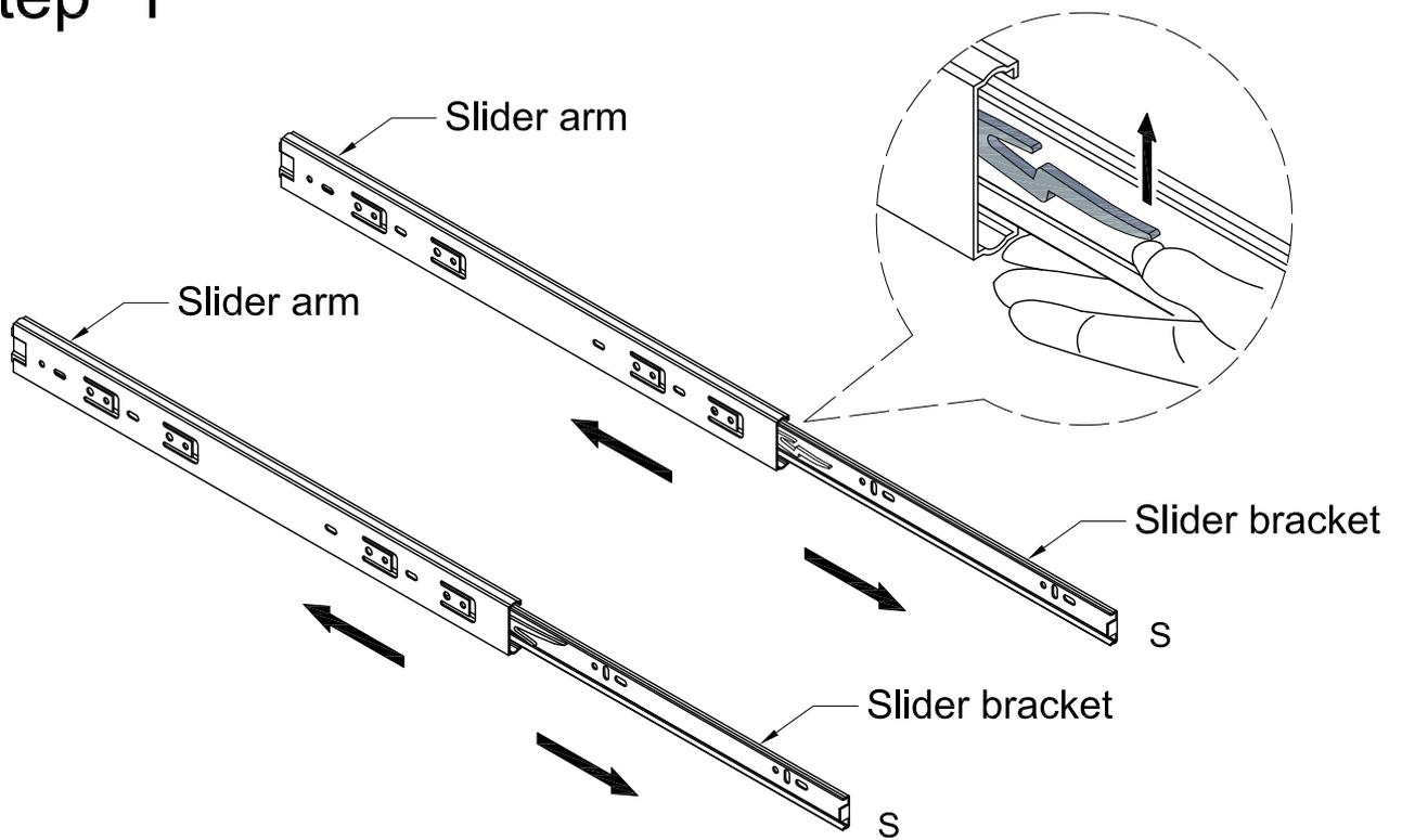
Disassemble drawer slider (S) by sliding the slider arm and slider bracket apart. Depress the small lever of the slider bracket and carefully pull the two pieces apart. Repeat this process for both drawer sliders (S).
