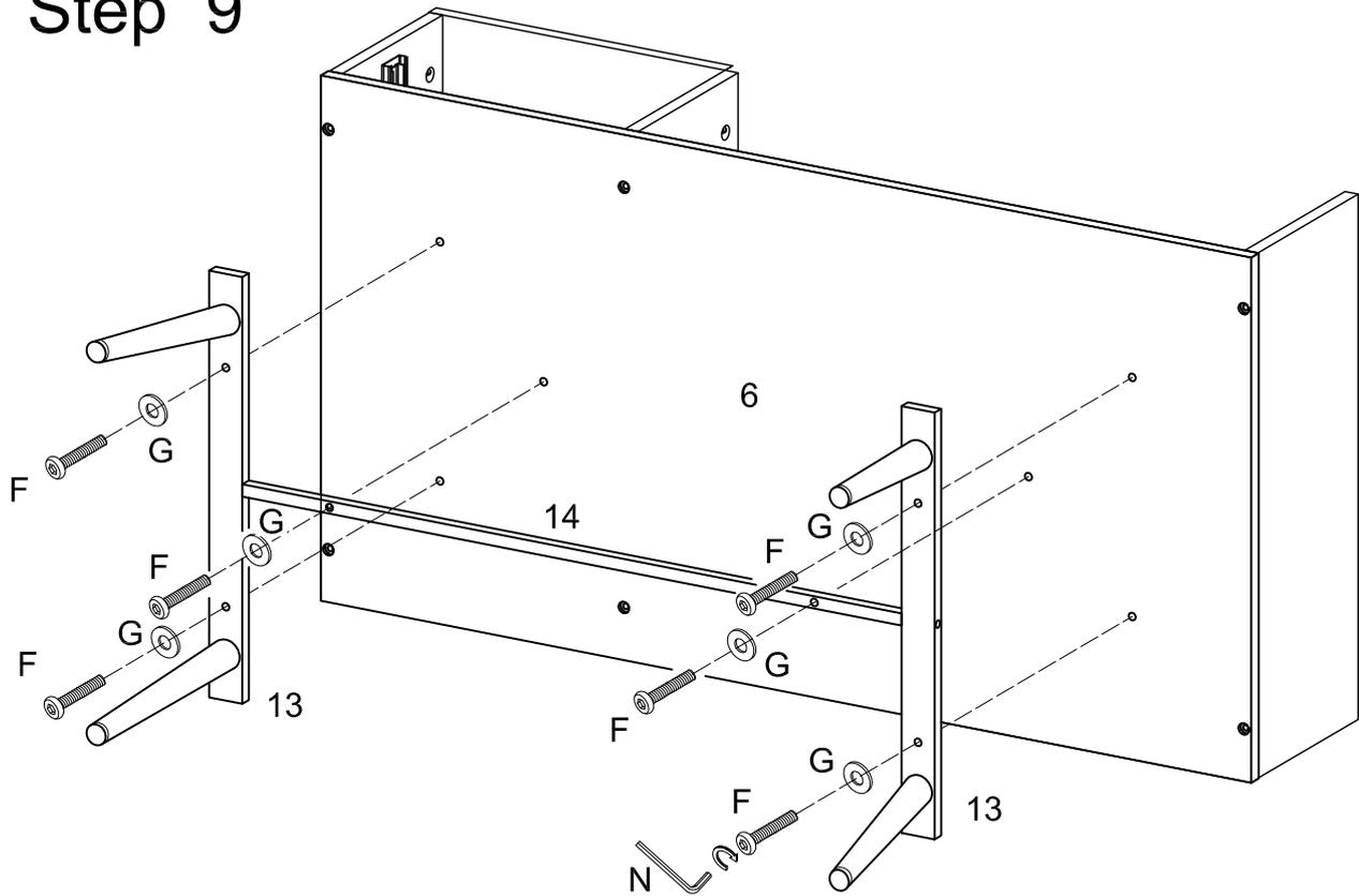
Use wrench (N) to secure leg (13) and part (14) to bottom panel (6) with bolt (F) and washer (G).
