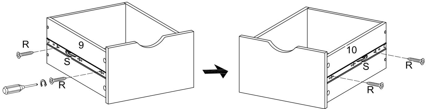
Secure slider bracket (S) to drawer side panel (9,10) with screw (R).
