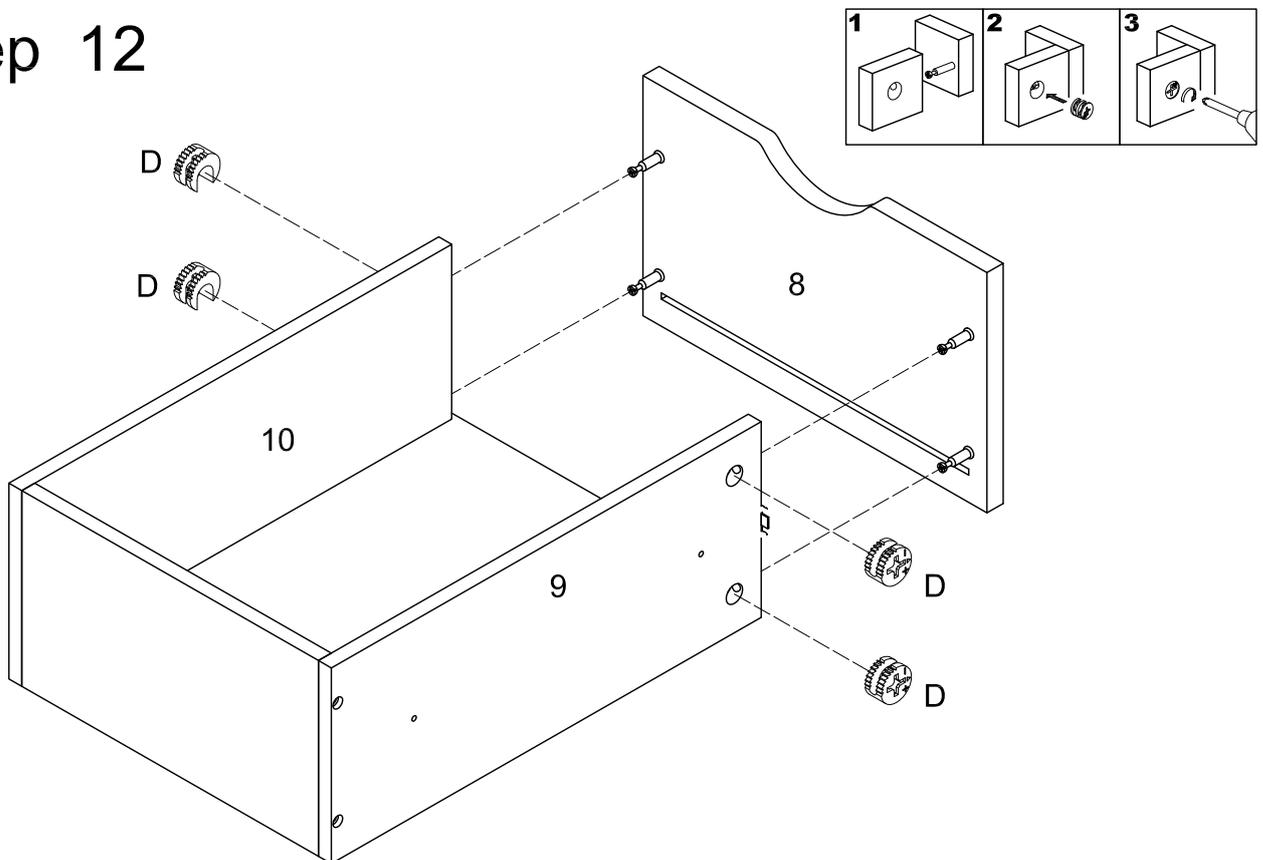
Insert drawer front panel (8) into drawer side panel (9,10), then insert and secure cam lock (D) to drawer side panel (9,10) to lock it.
