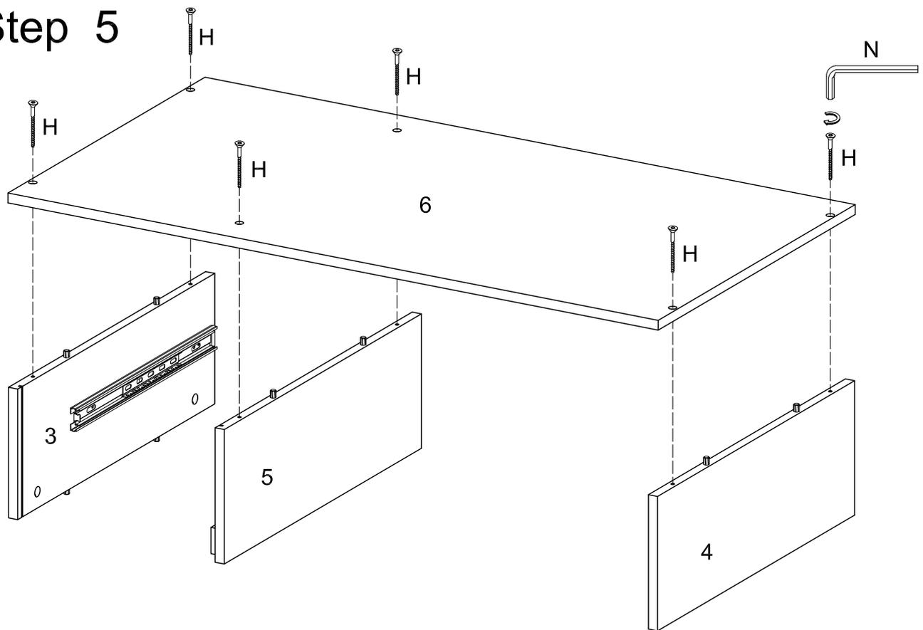
Use wrench (N) to secure bottom panel (6) to side panel (3,4,5) with bolt (H).
