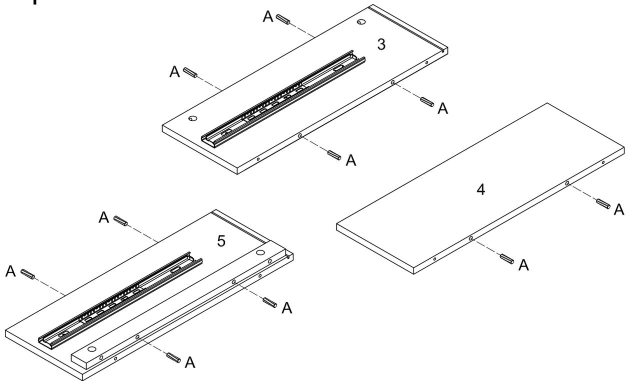
Insert wooden dowel (A) into side panel (3,4,5).
