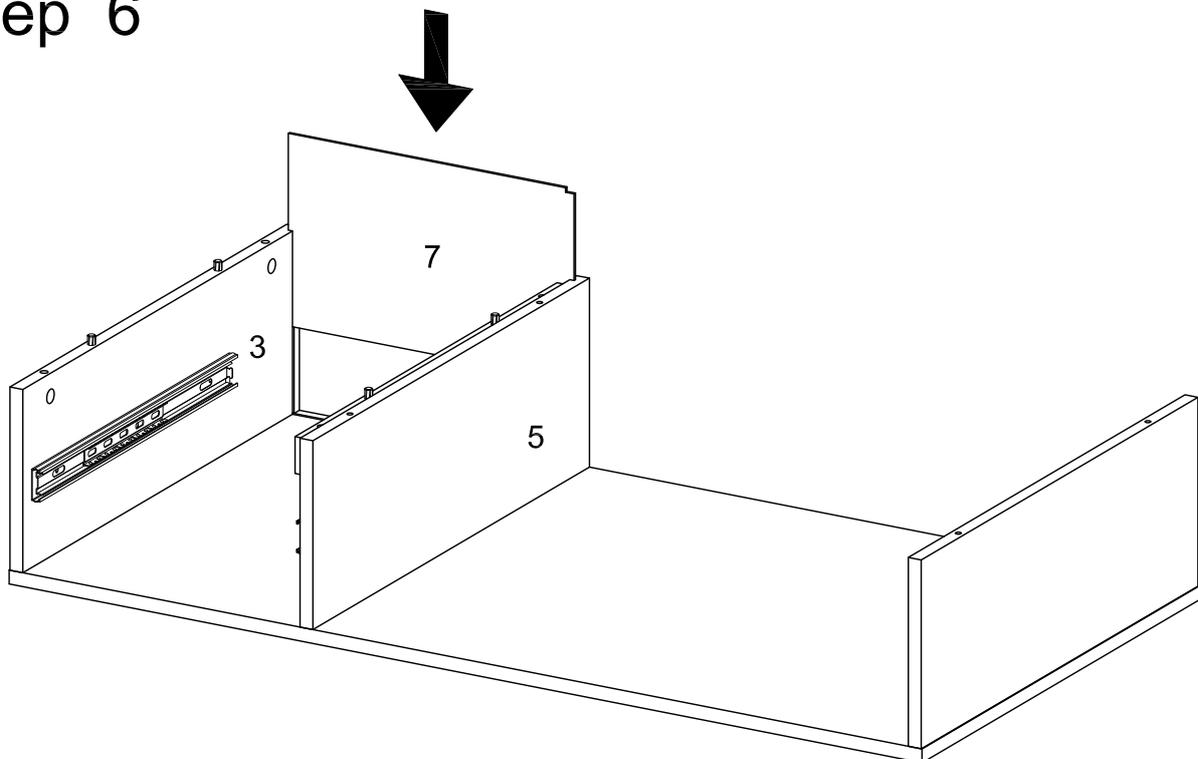
Slide back panel (7) into grooves as per diagram.
