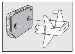
■ Fit the plinth filter back on the handle. Make sure it is the correct way round.
