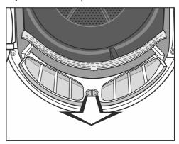
Hold the knob and pull the lint filter forward to remove it.
