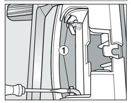
■ Insert the end of the screwdriver blade under rod ① and rotate it so it is in an upright position. Do the same to the other rod.
