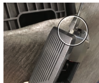
Connect the Power Supply Connector to the Power Supply
