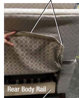
Rear Body Rail - Fastening Tape on Backside (not visible)
