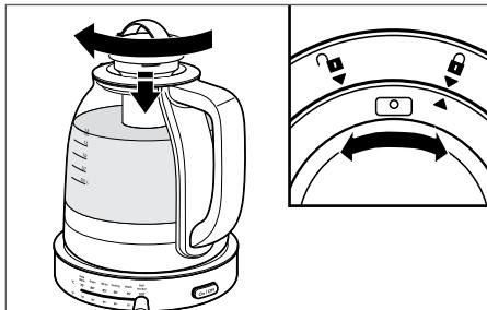
5. Place the tea steeper lid assembly inside the kettle lid. Twist the handle so that the tea steeper lid locks into place in the kettle lid. When locked into place, the indicator on the tea steeper lid will line up with the indicator next to the locked symbol on the kettle lid.
