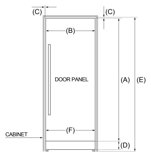
NOTE: The refrigerator comes with a 4" (100 mm) stainless steel toe kick installed to fit a standard 84" (2134 mm) tall cabinet niche. For flush installation in a standard 25" (635 mm) deep cabinet niche, maximum door panel thickness is 15/16" (24 mm).
