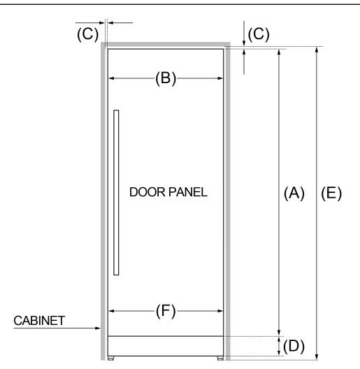
NOTE: The refrigerator comes with a 4" (100 mm) stainless steel toe kick installed to fit a standard 84" (2134 mm) tall cabinet niche.
