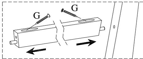
**STEP 3:** Attach the "H" stretcher to the front legs and chair back with wood screws (G). Completely tighten all wood screws and bolts. Turn the assembled chair to the upright position.
