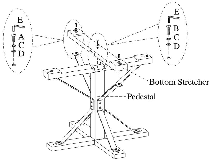
**STEP 5:** Put the table top upside down on a soft surface, and attach the pedestal assembly to the table top by using 4 bolts (B), lock washers (C) and flat washers (D) as shown below. Use the allen wrench (E) to tighten all bolts. Turn the assembled table to the upright position.
