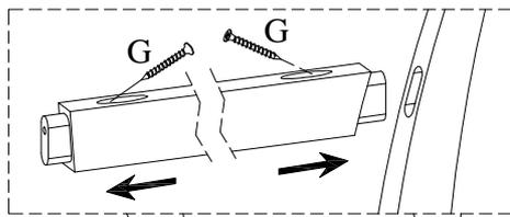
**STEP 3:** Attach the left side stretcher and right side stretcher to the front legs and chair back with wood screws (G). Completely tighten all wood screws and bolts. Turn the assembled chair to the upright position.
